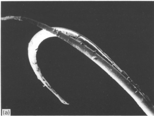
Figure 14 Tensile breaks of polyester fibres after flexing for limited periods: (a) 15 min, 45 000 cycles; (b) 15 min, 45 000 cycles.
