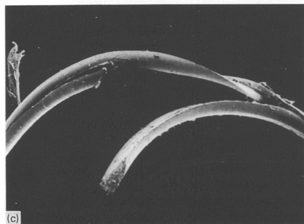
Figure 5 Progressive damage in nylon 6 fibres: (a) 5 min, 15 000 cycles; (b) 10 min, 30 000 cycles; (c) 15 min, 45 000 cycles; (d) 15 min, 45 000 cycles; (e) 15 min, 45 000 cycles; (f) 15 min, 45 000 cycles.
